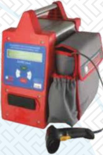
The electrofusion welding unit model Euro SP1 plus is a polyvalent unit suitable for the welding of all electrofusion fittings up to diameter d. 630. It allows to operator to work at safety voltage lower than 50 Volt, is manufactured according to UNI 10566 and ISO 12176- 2 standards, as well as provided with CE mark.
