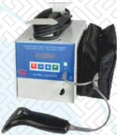
The electrofusion welding unit model Euro JUNIOR is a polyvalent unit suitable for the welding of all electrofusion fittings up to diameter d. 160. It allows to operator to work at safety voltage lower than 50 Volt, is manufactured according to UNI 10566 and ISO 12176-2 standards, as well as provided with CE mark.
