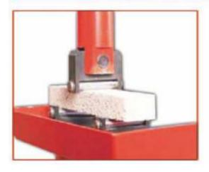
High compressive strength 2350 kPa required for a 2 cm thickness It is also resistant against impacts
